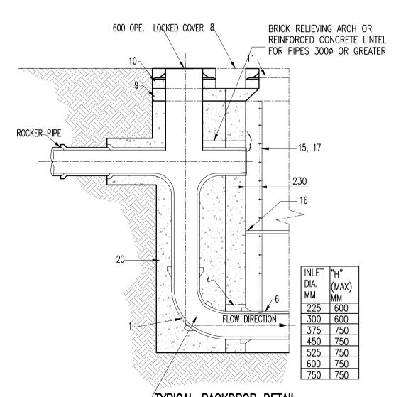
2NO. 45° BENDS FOR PIPES UP TO 375MMø 1 NO. 90° BEND FOR PIPES 450MMØ OR GREATER
